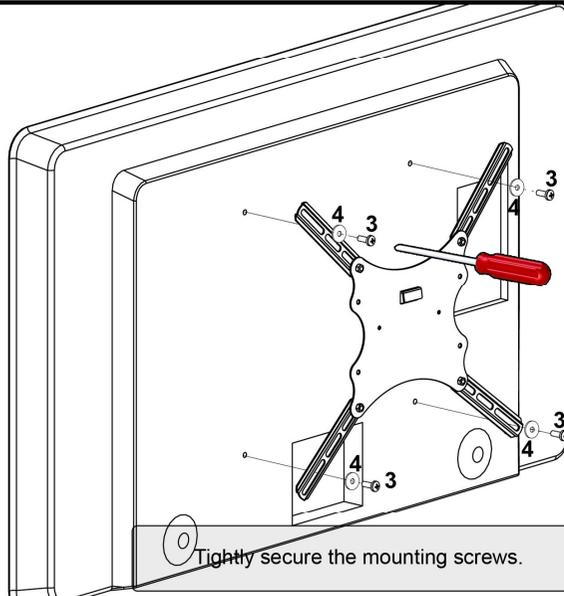
Tightly secure the mounting screws.
